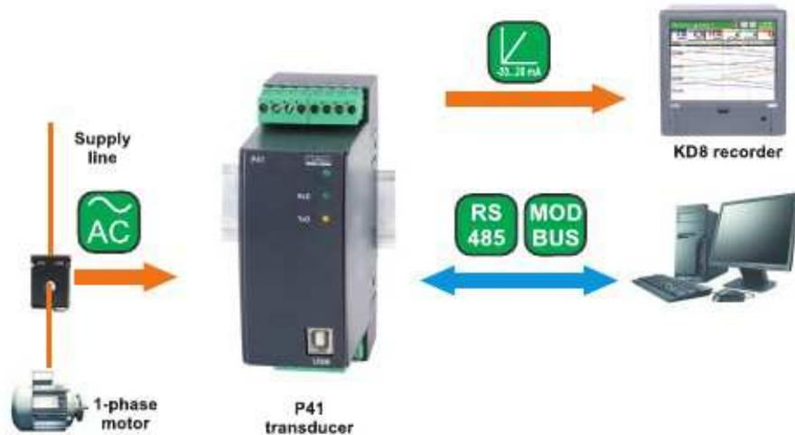
Conversion and recording of current engine load and energy consumption.
