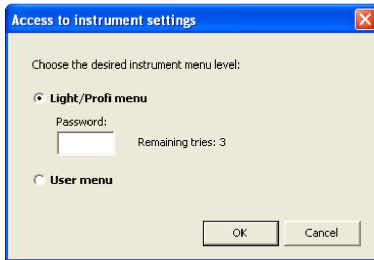
In the dialog box, you are supposed to choose the required level and, in the case of **Light/Profi menu**, to enter a password. (The appropriate level "Light" or "Profi" is then determined by the given password.)
