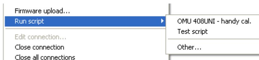
When you click one of the scripts from the list, the script is executed for the on-line connected instrument. The script runs in a separate window - **OM Script shell**, which provides the user interface defined inside the script. After the script gets started, follow the instructions in the shell window.
