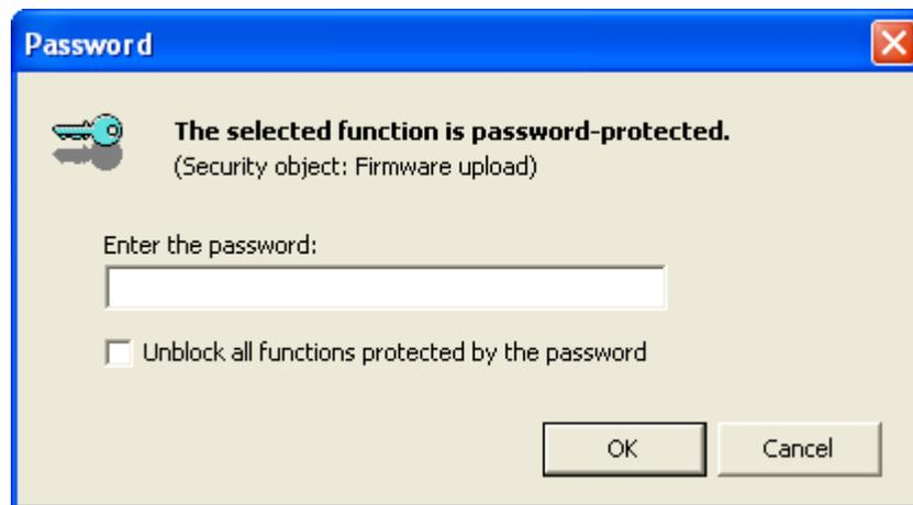
Enter the correct password to unblock the function. You can also check the box "**Unblock all functions protected by the password**", which causes that the application will not require the password again to any of the protected functions (till the application exit). Click the **OK** button for confirmation.
