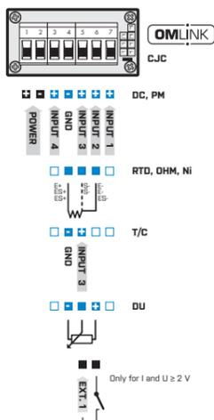
Power supply cord should not be near low voltage input signal leads. Contactors, large electrical motors and other power elements should not be operated in the vicinity of the instrument. Input signal leads (measured value) should be separated from all power devices. Our instruments are extensively tested and they comply with relevant standards for use in industrial environment, however, adhering to the above mentioned measures is strongly advised.
