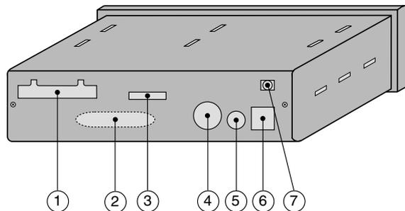
1. Parallel inputs, plug-in screw terminals.
