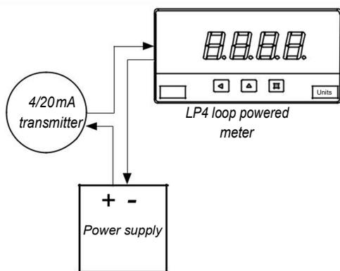
The LP4 loop powered meter can be used to for local visualization of the transmitter reading.
