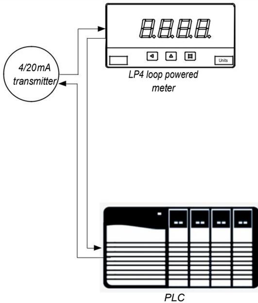
The LP4 loop powered meter can be directly inserted into the existing current loop that connects the transmitter and the PLC. Just cut the loop, and connect the LP4. Place it close to the transmitter to provide instant information to the local operator and maintenance personnel.
