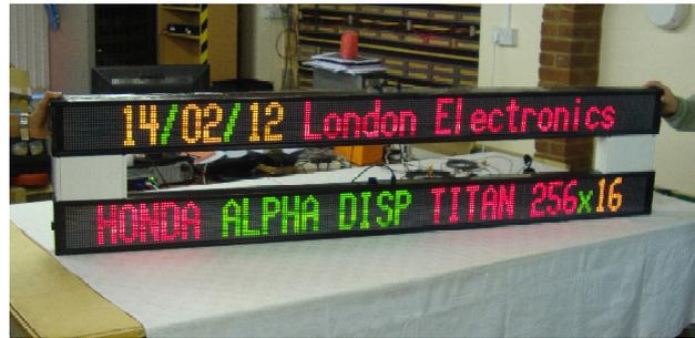
The Titan series is assembled from a combination of inter-connecting modules.
