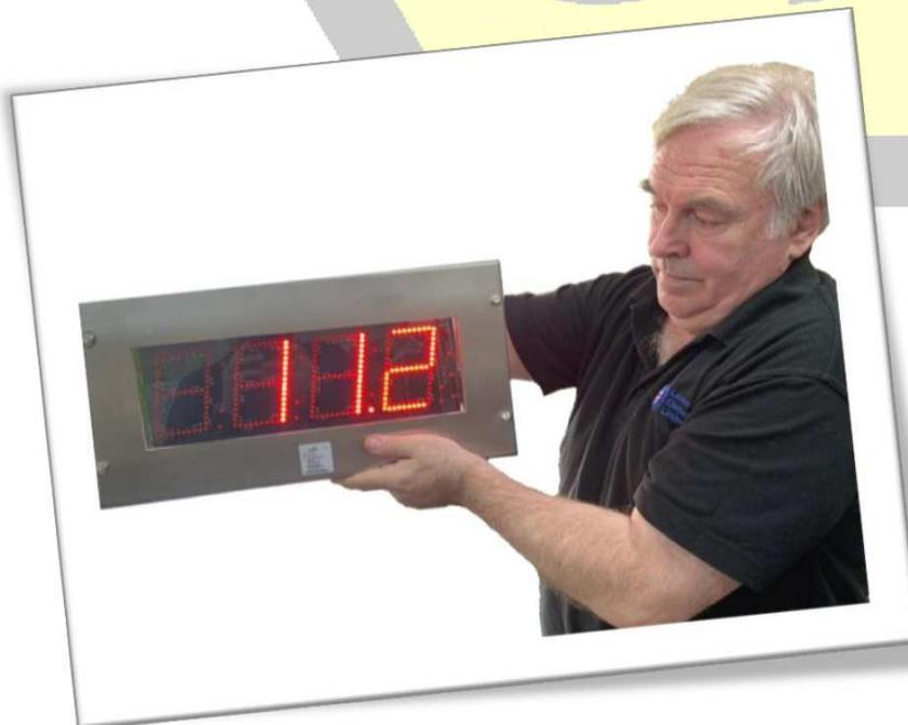
We manufacture the largest range of ATEX large digit displays on the market, like this display with 4 inch (102mm) high digits
