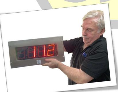
We manufacture the largest range of ATEX large digit displays on the market, like this display with 4 inch (102mm) high digits
